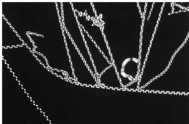
Figure 2. Microscopic texture of the B_7 phase exhibiting the spiral domains at 171.5^\circ\text{C} . Notice a small region (right of centre) where a myelinic texture is also seen. Magnification \times 320 .
